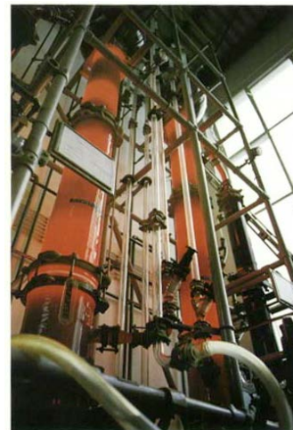
Photograph of the cylindrical immersion type reactors used by Dragoco for the production of (-)-rose oxide
